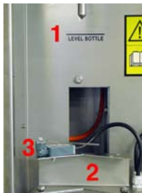
Figure 2. Top of bottle must be level with "LEVEL BOTTLE" line (1). Center bottle with nozzle by adjusting back support (2). Adjust microswitch (3) to insure it 'clicks' when bottle is placed on platform.
