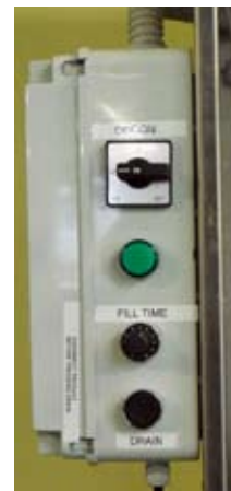
Figure 5. OFF/On switch at top with green indicator light below it. Fill Time adjustment. DRAIN button used only if product line is disconnected.
